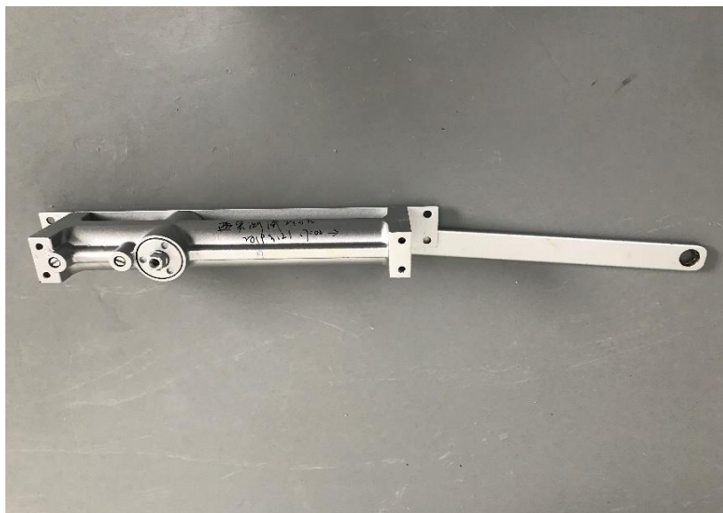
Front view (afte 240h salt spray test)
