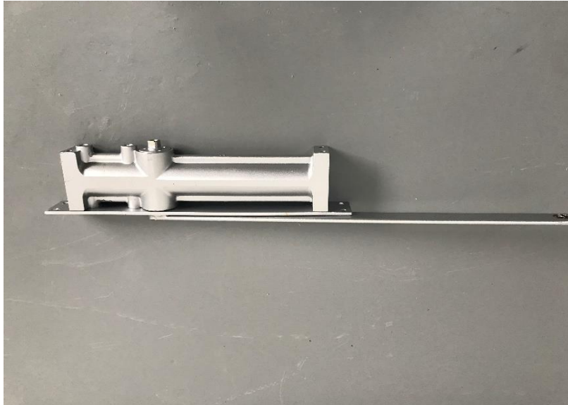
Section view (afte 240h salt spray test)
