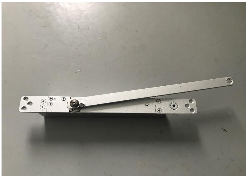
Front view (afte 240h salt spray test)
